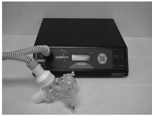
Figure 1. The CardioCoachCO 2 metabolic testing device.
